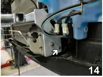
14. Insert 3/8-16 nut plates through the frame rail opening and align with the upper two drilled holes. Insert 3/8-16 x 1 1/2" hex bolts and 3/8" lock washers and tighten to the 3/8-16 x 1" hex bolt into the bottom hole (see arrow in photo above) and fasten to the 3/8-16 hex nut and 3/8" lock washer. Do this to both sides of the vehicle.
