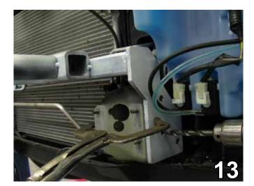
13. Using the baseplate as a template, drill three holes into the frame rail with the 13/32" drill bit. Do this to both sides of the vehicle.
