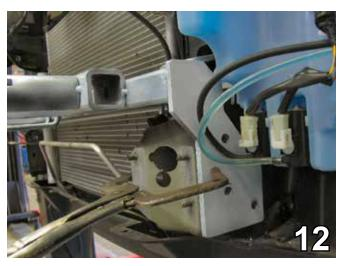
12. Align baseplate so that it is flush with the bottom and front edge of the frame rail. Clamp the baseplate in place with the large vise grips. Do this to both sides of the vehicle.
