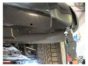
5. Remove three Phillips screws from the bottom of the fascia. Two are found just forward of the front tires, on both sides of the vehicle, another is in the center of the fascia. The photo above only shows the screw forward of the front tire on the driver's side. Set all bolts aside to be reinstalled later.
