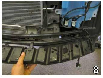
8. Pull forward on the plastic pieces clipped to the metal bumper. Do this to both sides of the vehicle. Set plastic clips aside to be reinstalled later.
