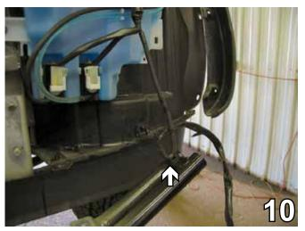
10. Pull bumper forward. Wire clips are still attached to both sides of the metal bumper. Remove these with a pushpin puller to release the metal bumper. Set bumper aside to be reinstalled later.
