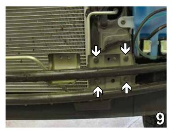
9. Using a 12MM socket, remove four metric bolts from the metal bumper. Do this to both sides of the vehicle. Set bolts aside to be reinstalled later.
