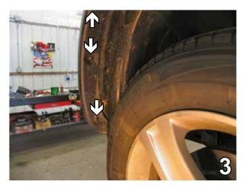
Just forward of the front tire, inside the wheel well, remove three Phillips screws. Begin with the screw at the bottom of fascia and work upward, removing two more. Do this to both sides of the vehicle. Set screws aside to be reinstalled later. Top Phillips screw is not shown.
