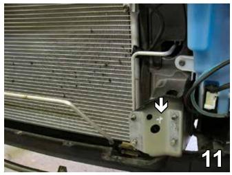
11. Using a 1 1/4" hole saw, cut a hole in the front of the frame rail to open up an area for the nut plate. Do this to both sides of the vehicle.
