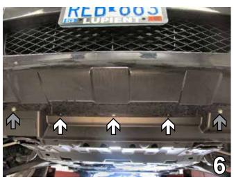
6. Remove six pushpins from the bottom of the fascia, pushpins are indicated by the white arrows in the photo above. Using a 10MM socket, remove two metric bolts, as indicated by the grey arrows in the photo. Arrows in graphic do not indicate all the pushpins that will be removed, but show where bolts and pushpins can be found.
