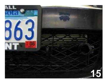
15. Align the fascia to its original position and, using a diagonal cutter, trim necessary openings in the grille for the attachment tabs, convenience links, and electrical rods.
