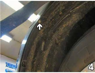
Using a 10MM socket, remove one metric bolt just below the last Phillips screw removed. Do this to both sides of the vehicle. Set screws aside to reinstall later.
