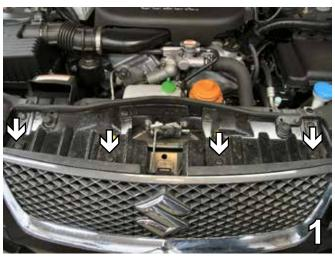
Remove four pushpins from behind the grille. Set pushpins aside to be reinstalled later.
