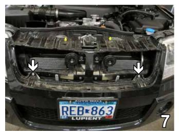
7. Using a 10MM socket, remove two metric bolts from the fascia between headlights and just behind the grille removed earlier. Pull fascia forward, disconnect the fog lights on both sides of the vehicle. Also disconnect the temperature sensor found on the driver's side. Set bolts and fascia aside carefully to be reinstalled later.
